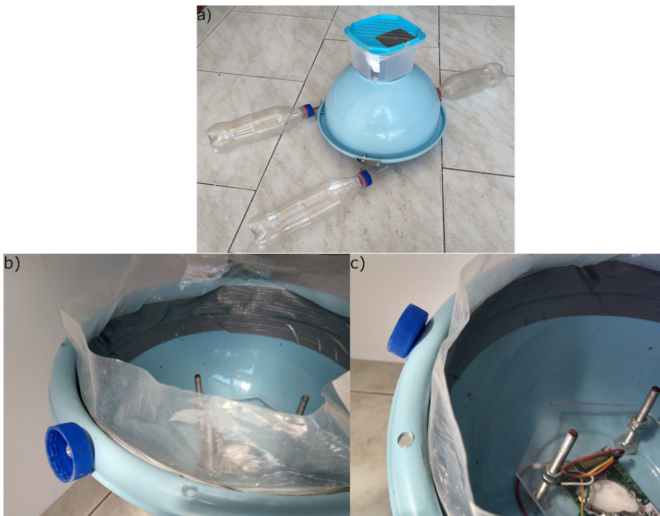
Figure C1. Overview of the Flexible Foil chamber (panel a). Close up on the support of the floating system (panel b). Protection of the sensor from the water droplets (panel c).
