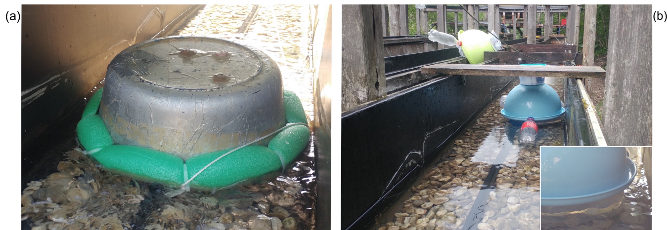
Figure 1. Two chambers design: on panel (a) the Standard chamber from Bastviken et al. (2015) instead on panel (b) the Flexible Foil chamber (with a close-up of the peculiarity of the sealing).
