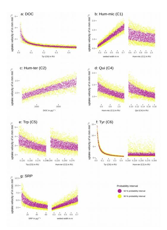
Figure 7: Simulated change of uptake velocity  $v_f$  with variation of one parameter Table 1. The colours show the 50 % (violet) and the 90 % (yellow) percentile intervals.
