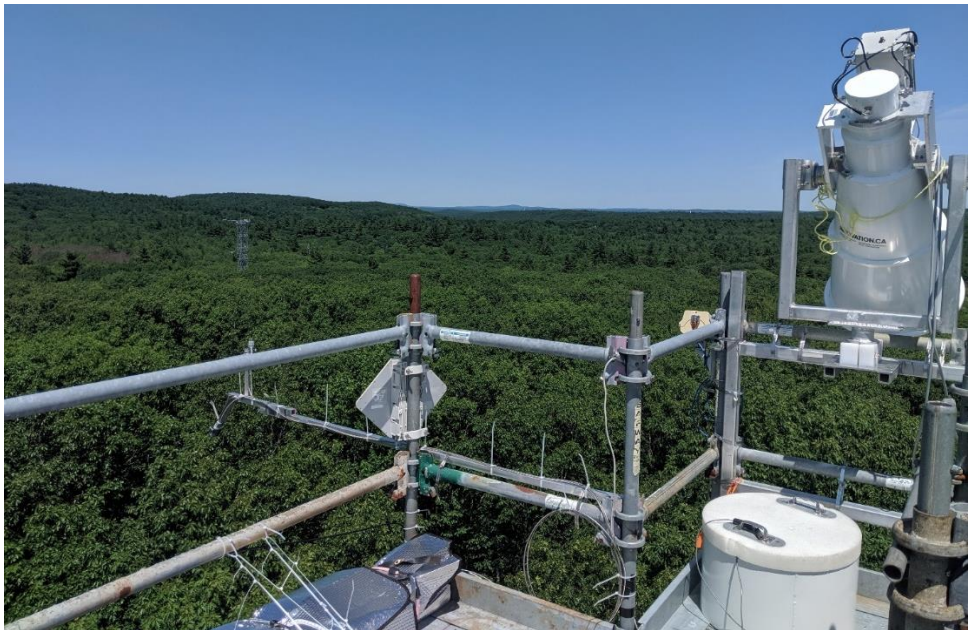
Figure 1. Radiometer setup at Harvard Forest hardwood walk-up tower.
