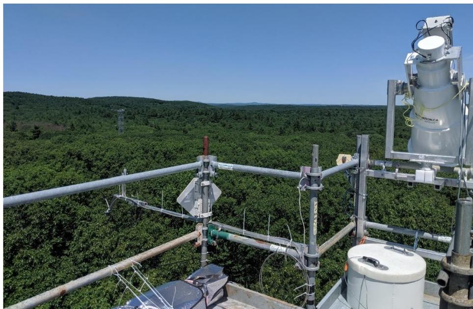
115 **Figure 1. Radiometer setup at Harvard Forest hardwood walk-up tower.**
