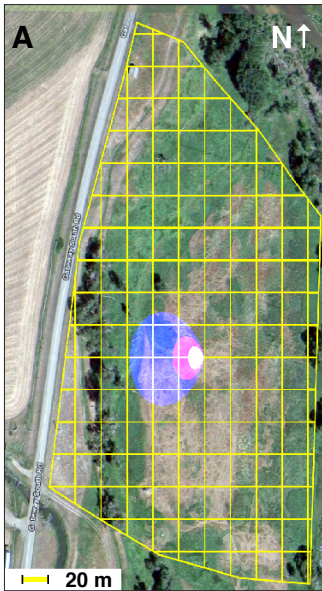
Figure 3: An eddy covariance flux footprint calculated following (A) Hsieh et al. (2000) extrapolated to two dimensions following Detto and Katul (2006) and (B) Kljun et al. (2015) for a single 30-minute interval superimposed on the study field (Figure 1). The purple, pink, and white areas represent the 95%, 75%, and 50% footprint during 1030 AM – 1100 AM Mountain Standard Time on January 8, 2018. The fraction of the footprint in each grid box is summed for each 20-m pixel to calculate the contribution of each pixel to the total flux. Background image: Google, Maxar Technologies and the USDA Farm Service Agency ©2018.
