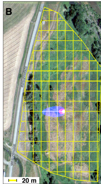
Figure 3: An eddy covariance flux footprint calculated following (A) Hsieh et al. (2000) extrapolated to two dimensions following Detto and Katul (2006) and (B) Kljun et al. (2015) for a single 30-minute interval superimposed on the study field (Figure 1). The purple, pink, and white areas represent the 95%, 75%, and 50% footprint during 1030 AM – 1100 AM Mountain Standard Time on January 8, 2018. The fraction of the footprint in each grid box is summed for each 20-m pixel to calculate the contribution of each pixel to the total flux. Background image: Google, Maxar Technologies and the USDA Farm Service Agency ©2018.
