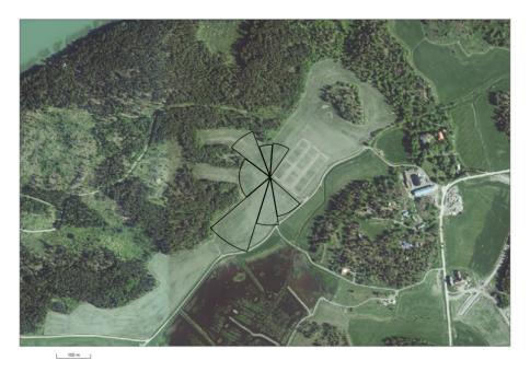
**Figure 1.** Experimental field with the sectors representing the target area. the area covers 3.9 ha. Eddy covariance tower is located in the centre of the sectors. Wind directions from 30 to  $140^{\circ}$  were filtered out due to another experimental plot locating in that part of the field. (Orthophoto from National Land Survey of Finland)
