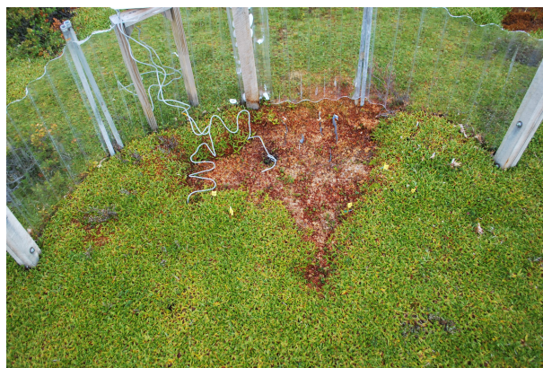
Figure 2. Experimental setup. Open side chamber (OSC), open to the north, installed in an Astelia pumila (light green color) cushion with a patch of Sphagnum magellanicum (reddish-brownish color)
