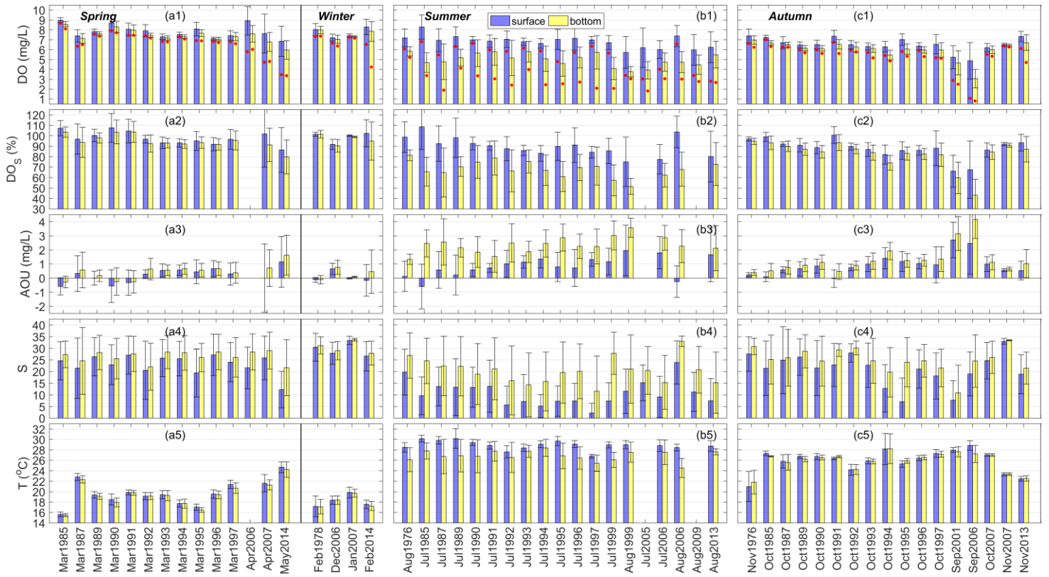
715 Figure 2. Spatial means and standard deviations of DO concentrations, DO saturation (DO s ), apparent oxygen utilization (AOU) , salinity (S), and temperature (T) in the surface and bottom waters of the PRE in (a) spring (March-May) and winter (December-February), (b) summer (June-August), and (c) autumn (September-November) during 1976-2014. Note that the red dots in the first row of the figure represent the lowest DO values measured in each time period.
