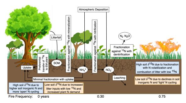
Figure 1. Conceptual diagram of processes influencing wood  $\delta^{15}$ N values at the CCESR burn experiment. Fractionation against <sup>15</sup>N occurs with transformations of plant-available N in soil and gaseous N loss. Colored boxes indicate potential contrasting effects of fire frequency on soil  $\delta^{15}$ N values. Blue and orange boxes indicate processes leading to higher and lower relative soil  $\delta^{15}$ N, respectively. Graphic adapted from (van der Sleen et al., 2017).
