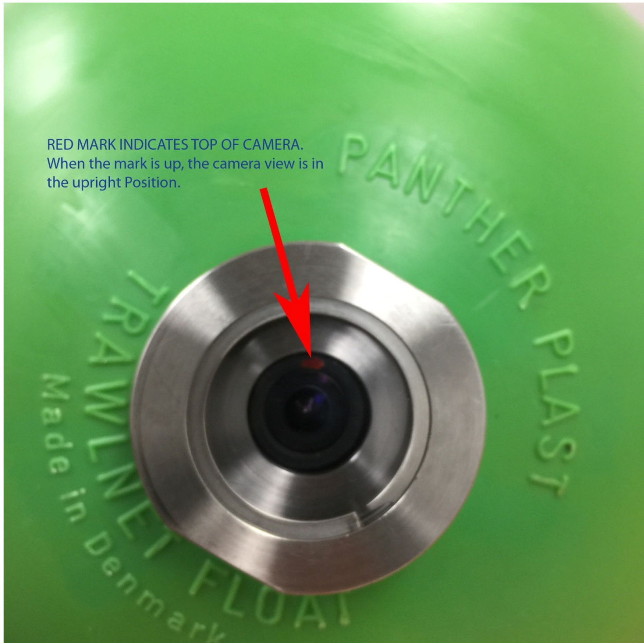
Figure 4 The window port located on the bottom of the camera hemisphere. The red mark on the lens indicates the upright position.
