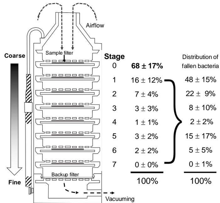
**Figure S5-1.** Percentages of residual bacterial cells after the sampler was run for 24 h. If no bacteria fall from the top stage, the percentage in bold should be nearly 100%. The actual percentage was 68%, indicating that 32% of the bacteria fell from the top stage. The distribution of fallen bacteria is shown in the right column. The fallen bacteria were mostly in the second and third stages and did not affect the lower stages of the sampler.
