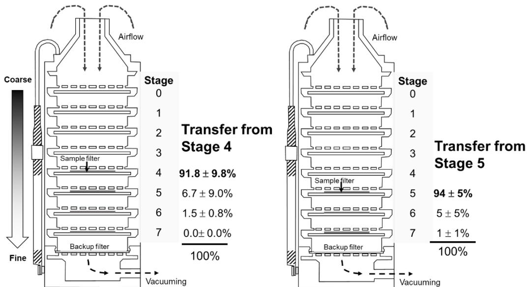
**Figure S5-2.** The distribution of bacterial cells fallen from Stage 4 (left) and Stage 5 (right) to lower stages. Averagely less than 10% of the bacteria fell from the original filters in Stage 4 or 5 to lower stages.
