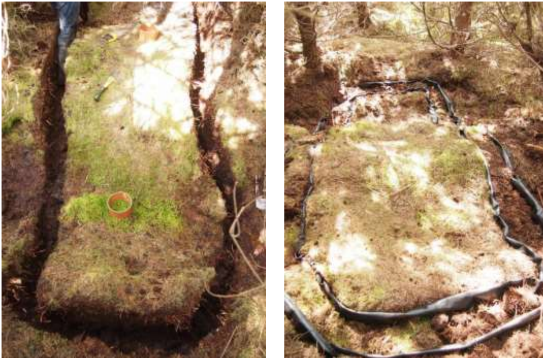
Figure 2 Left: trenching plot dug and all living tree roots are sawn trough. Right: finished trench plot; trenches double lined with polypropylene gardening cloth and filled in with peat.
