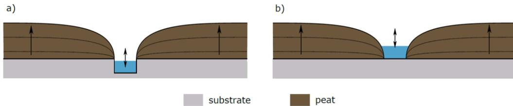
315 **Figure 8: Sketch of the two conceptual channel models used for the long-term peatland development simulations. a) Rectangular channel, situated within the substrate, with the top of the channel corresponding to the base of the peat. b) The channel located on top of the substrate, with the channel bottom corresponding to the base of the peat. The channel walls consist of the sloping sides of the peat bodies.**
