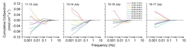
Figure 7. Change of the cumulative co-spectra for the 3S  $O_2$  flux during the deployment week. Cumulative co-spectra were calculated for hourly intervals from 16:00 to 24:00 for the four deployment periods (0.12 nmol cm<sup>-2</sup> s<sup>-1</sup> corresponds to 4.3 mmol m<sup>-2</sup> h<sup>-1</sup>). Colors indicate the time periods for which the co-spectra were calculated.
