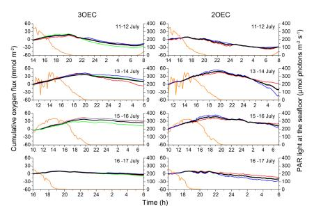
Figure 4: Comparison of 3OEC and 2OEC fluxes. Cumulative fluxes for July 11-12, 13-14, 15-16 and 16-17 (top to bottom) with the respective light (PAR) intensities (orange lines) at the seafloor for 3OEC (left column) and 2OEC (right column). Sensor 1: red, Sensor 2: blue, Sensor 3: green, average sensor signals: black thick lines.
