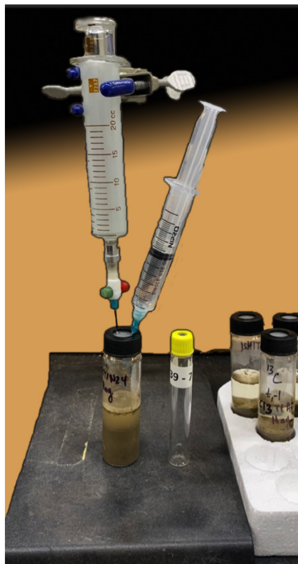
Supplemental Figure S1. Typical sampling setup (All Experiments). A gas tight syringe was inserted first, relieving the excess pressure and recording the volume of biogenic gas produced. With the pressure was equalized to 1 atmosphere, a separate syringe was used for gas and liquid sampling. If desired, an inert gas (e.g. nitrogen) may be injected into the headspace, up to the gas tight syringe volume, prior to sampling. The experiment was performed in 1-liter jars (left) and we used the same gas and liquid sampling technique shown here with in 40 mL VOA vials (right). The liquid height in the jars was sufficient for liquid sampling with a 3" syringe.
