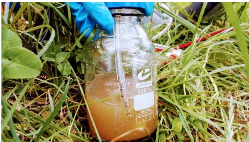
Figure 2. Bubbling water samples to measure dissolved gas concentration of \text{CH}_4 and \text{CO}_2 .
