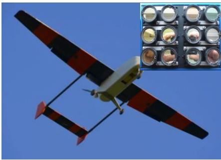
Figure 2: Unmanned Aerial System (UAS) Carolo P360 with multi-camera array Mini-MCA 12 (visible lenses at the underside of the camera).
