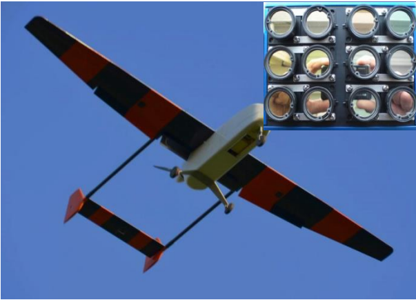
Figure 2: Unmanned Aerial System (UAS) Carolo P360 with multi-camera array Mini-MCA 12 (visible lenses at the underside of the camera).
