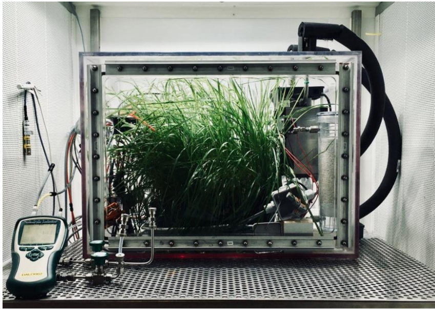
179 Fig.1. A vegetation-soil-atmosphere analog of the terrestrial biosphere in a closed chamber. (a) 180 Schematic of the closed chamber setup used for the terrestrial biosphere model. The 120 dm 3 liters 181 gas tight closed chamber containing a terrestrial biosphere analogue is enclosed in a larger growth 182 chamber from the Ecotron MicrocosmsMicrocosms platform. Main environmental parameters inside 183 the closed chamber are actively controlled and monitored: temperature (T), light intensity, CO 2 , 184 relative humidity (RH), pressure differential ( \Delta P ). The water cycle in the closed chamber is shown in 185 blue. (b) Photograph of the closed chamber used in the experiment with Festuca arundinacea .
