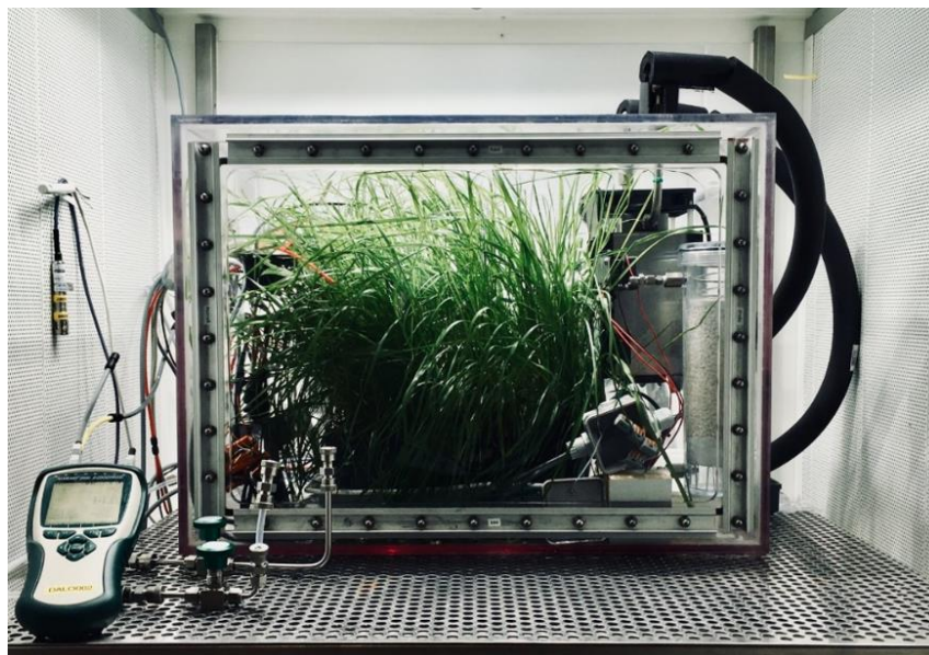
167 Fig.1. A vegetation-soil-atmosphere analog of the terrestrial biosphere in a closed chamber. (a) 168 Schematic of the closed chamber setup used for the terrestrial biosphere model. The 120 dm 3 gas 169 tight closed chamber containing a terrestrial biosphere analogue is enclosed in a larger growth 170 chamber from the Ecotron Microcosms platform. Main environmental parameters inside the closed 171 chamber are actively controlled and monitored: temperature (T), light intensity, CO 2 , relative humidity 172 (RH), pressure differential (ΔP). The water cycle in the closed chamber is shown in blue. (b) Photograph 173 of the closed chamber used in the experiment with Festuca arundinacea .
