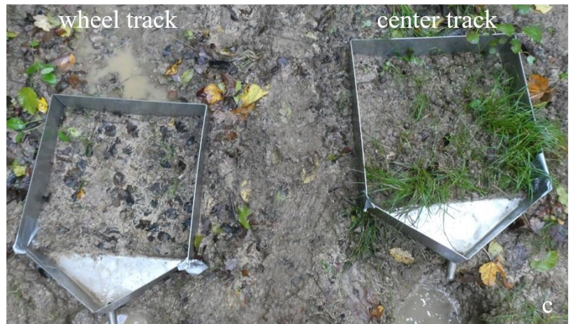
Figure A2: Experimental setup: a) Tübingen rainfall simulator inside the protective tent, b) Skid trail in the Trossingen-Formation (TS) in July 2019, c) Runoff plots in the wheel track and the center track in the Angulatensandstein-Formation (AS) in October 2019
