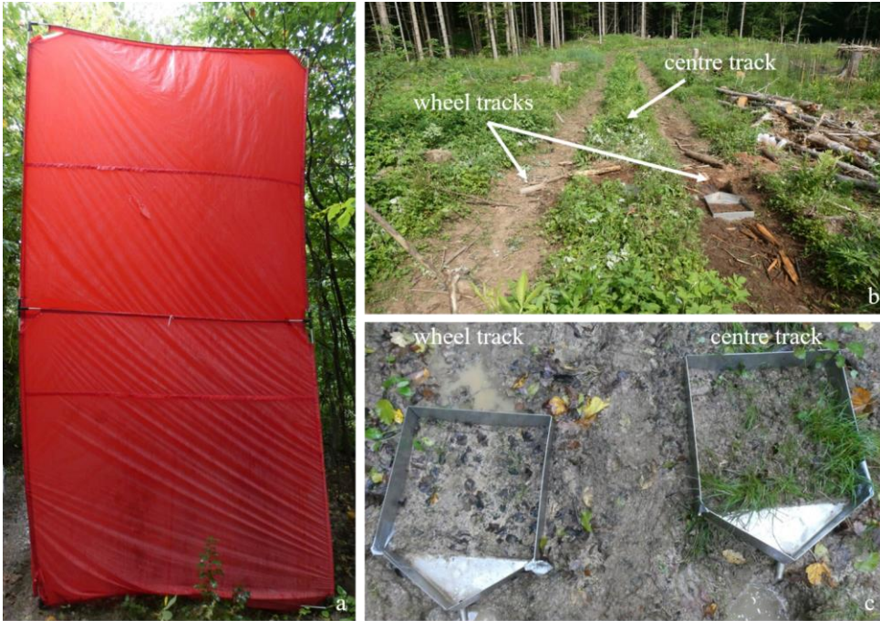
Figure A2: Experimental setup: a) Tübingen rainfall simulator with inside the protective tent, b) Skid trail in the Trossingen-Formation (TS) in July 2019, c) Runoff plots in the wheel track and the centre track in the Angulatensandstein-Formation (AS) in October 2019
