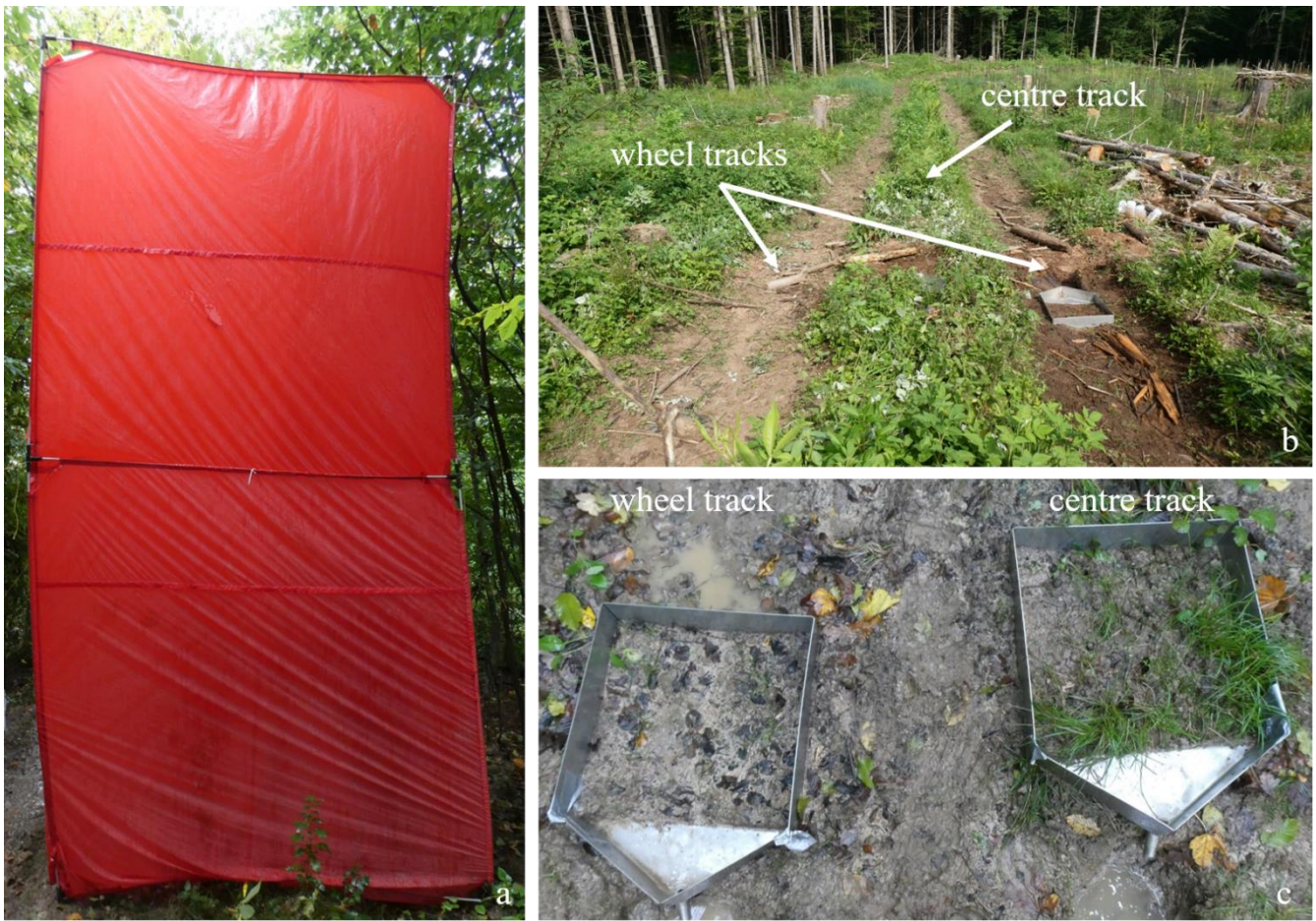
525 Figure A2: Experimental setup: a) Tübingen rainfall simulator inside the protective tent, b) Skid trail in the Trossingen Formation (TS) in July 2019, c) Runoff plots in the wheel track and the centre track in the Angulatensandstein Formation (AS) in October 2019
