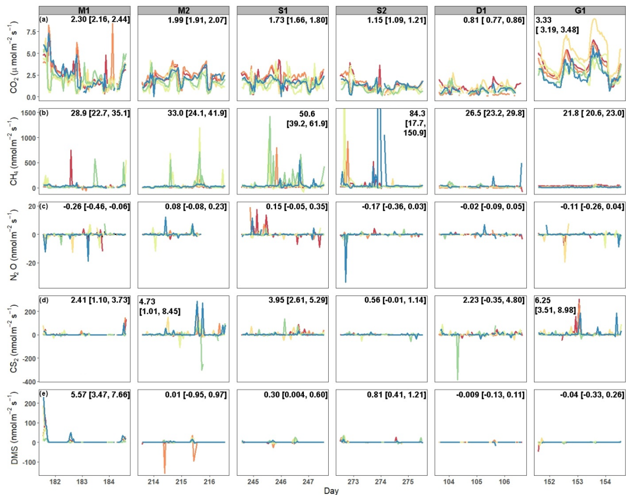
278 Figure 2. Time series of fluxes from each chamber during each campaign for (a) CO 2 , (b) CH 4 , 279 (c) N 2 O, (d) CS 2 , and (e) DMS. Each color designates a different chamber. The campaign means 280 [LCI = lower 95% confidence interval, UCI = upper 95% confidence interval] are listed on each 281 panel. The y-axis for CH 4 fluxes was shortened to show the variability. Full range of CH 4 fluxes 282 during S2 can be seen in Supplementary Figure (SF) 1.
