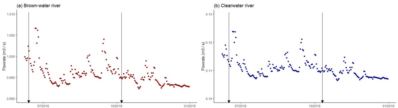
**Fig. S2** Estimated water discharge in (a) brown-water and (b) clearwater river determined based on the continuous pressure sensor data and measurements of the flow rate, cross section and water depth in June and October 2018. Arrows represent the sampling occasions.
