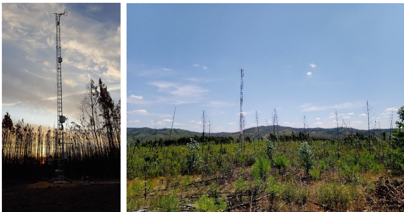
Figure 1: 12 m slim tower with eddy-covariance system at the burnt Pinus pinaster plantation (left: Photograph: J.J. Keizer, 22 September 2017) and the plantation after the windthrow (right: Photograph: J.J. Keizer, 20 June 2020)
