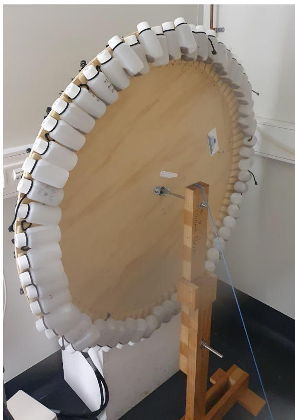
42 Figure S2. The plankton wheel used for experiments 1, 2, and 3. The picture shows the 43 plankton wheel with incubation bottles mounted on it.
