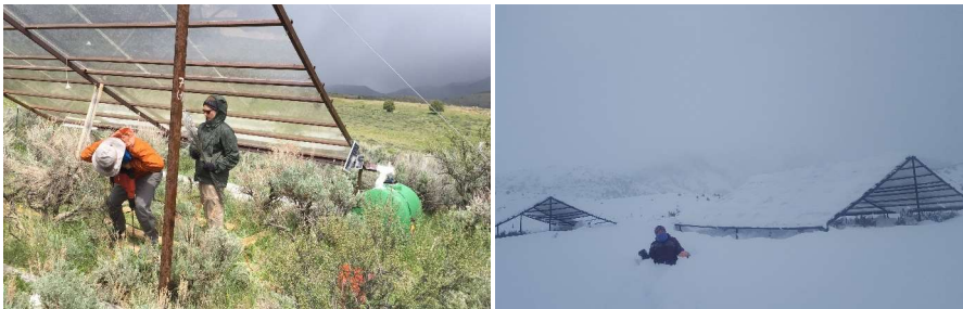
Fig. 1. Eleven precipitation manipulation shelters (8 m x 8 m) with plastic roofs collected and redeposited precipitation through as sprinkler system (a) and shovelingshovelling (b) as fewer, larger events. Tracer injections (a) were performed in plots to describe active root distributions of forbs, grasses and shrubs. Treatments were applied between spring 2016 and fall 2020 and
