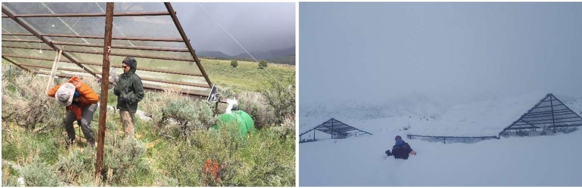
**Fig. 1.** Eleven precipitation manipulation shelters (8 m x 8 m) with plastic roofs collected and redeposited precipitation through a sprinkler system (a) and shovelling (b) as fewer, larger events. Tracer injections (a) were performed in plots to describe active root distributions of forbs, grasses and shrubs. Treatments were applied between spring 2016 and fall 2020 and vegetation growth measurements continued through 2021, one year after treatment removal.
