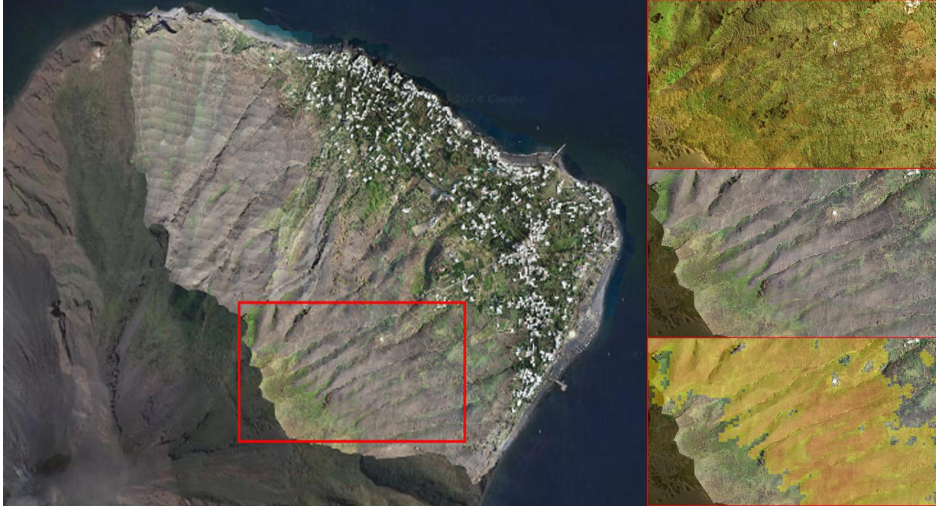
695 696 Figure 4: (left) high resolution drone image acquired on 17 August 2022 to assess the quality of the information derived from dNBR 697 analysis, overlaid on an high resolution image from Google Earth basemap; (top right) pre-fire detail from Google Earth basemap; 698 (middle right) post-fire detail from drone image; (bottom right) same detail with overlaid thresholded dNBR values higher than 0.19 699 (using pre-fire and August 2022 scene), semitransparent for visual comparison (yellow: low-, orange: middle-, red: high- severity 700 damage). Credits of drone images: Antonio Zimbone. Credits for Google base map: © 2024 Airbus, CNES/Airbus, European Space 701 Imaging, Maxar Technologies. 702 703 704
