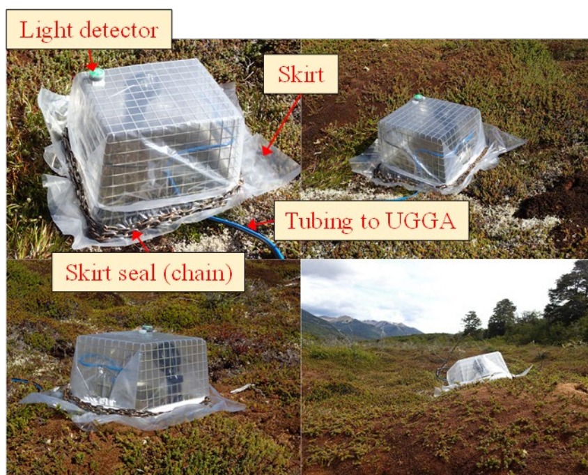
Figure S1: Photographs of the skirt-chamber under different configurations.
