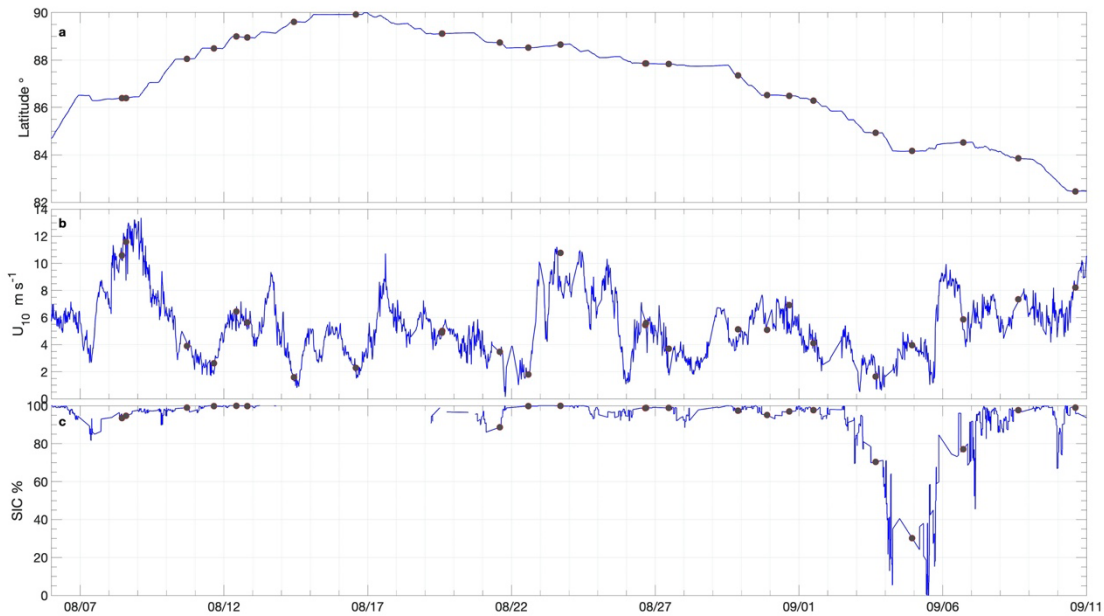
Figure 2. Time series of: a) Oden's latitude; b) wind speeds as measured on Oden ; c) SIC determined from the ASI 6.25km 2 product interpolated to Oden's position. Grey circles in each plot show averaged values corresponding to the times of flux chamber measurement.
